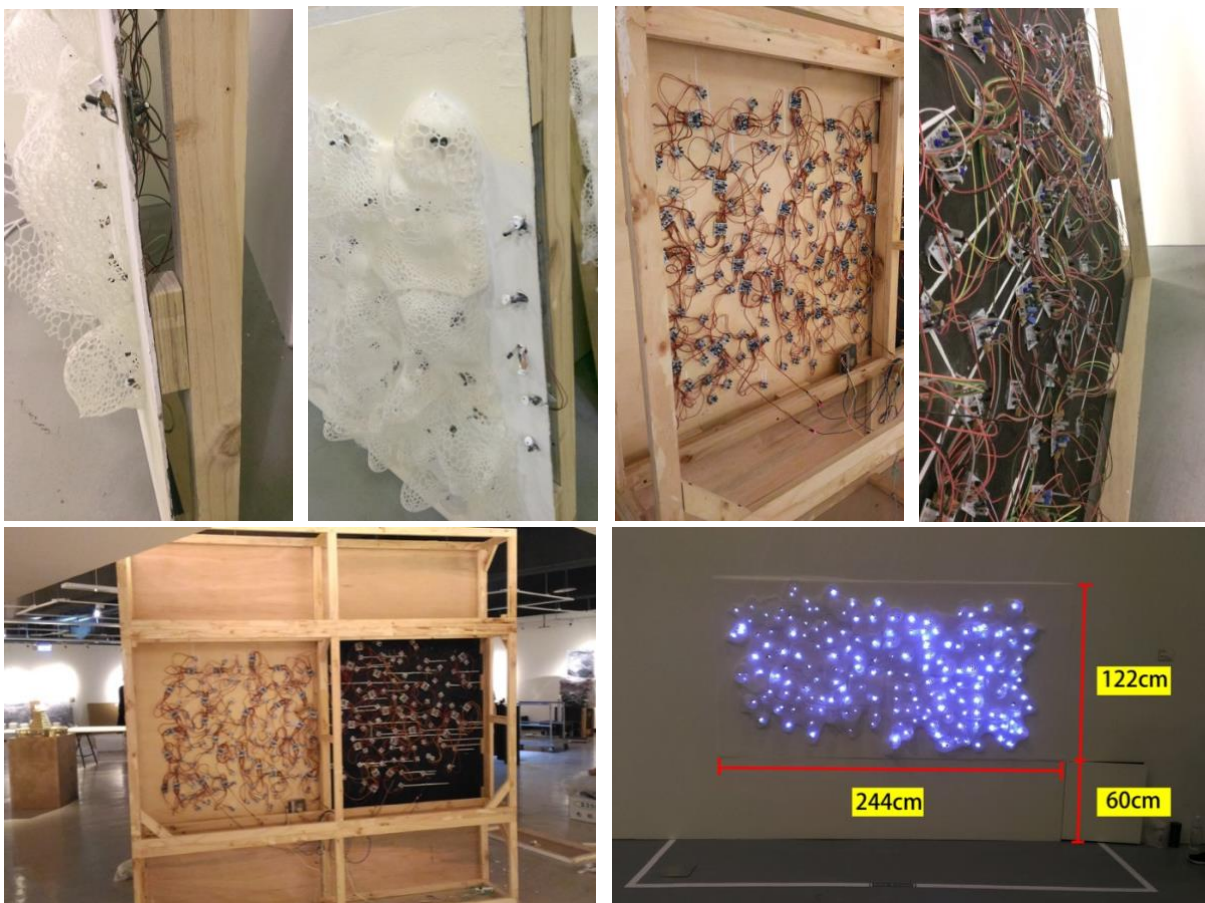
Figure 12. The figure shows the construction of PCB boards and wires behind the installation as well as the 3D-printed structure fixed on the front.
